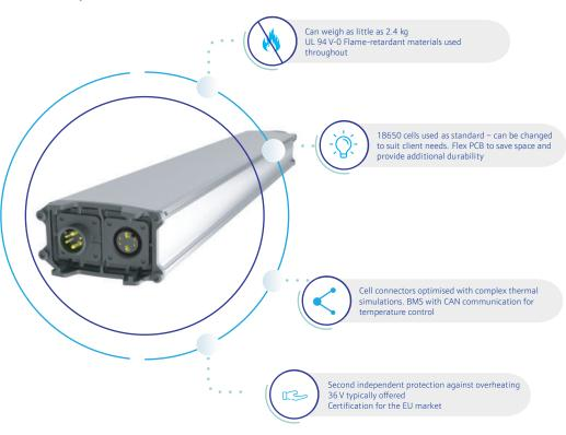
We understand that different clients will have different requirements, which is why we can offer full customisation of mechanics, electronics, and product configuration, such as cell model and IP rating.
